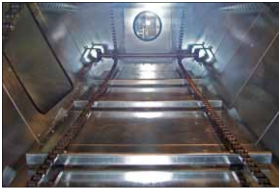
The photo to the left shows the inside of an Aagaard chain filter hopper.
